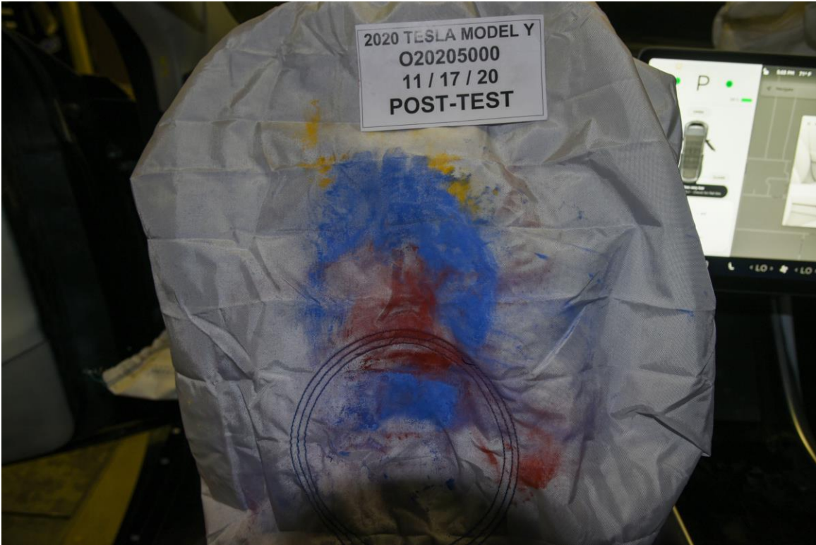
FIGURE 49. Post-Test Driver Dummy Contact with Airbag
