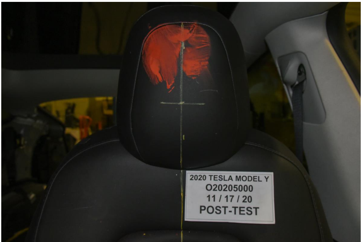
FIGURE 50. Post-Test Driver Dummy Contact with Headrest
