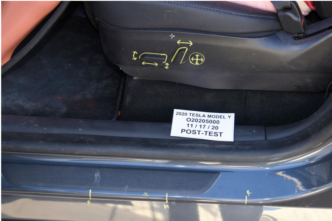
FIGURE 37. Post-Test Driver's Seat Fore-Aft Markings
