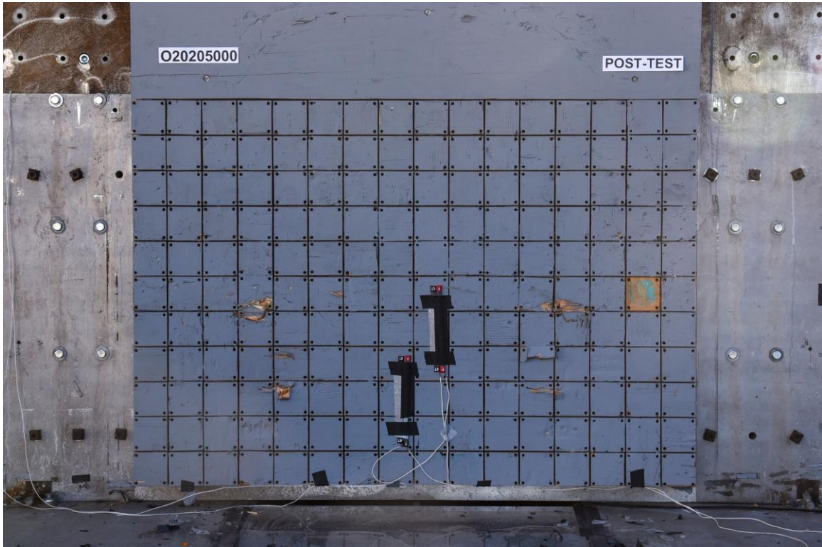
FIGURE 3. Post-Test Load Cell Wall
