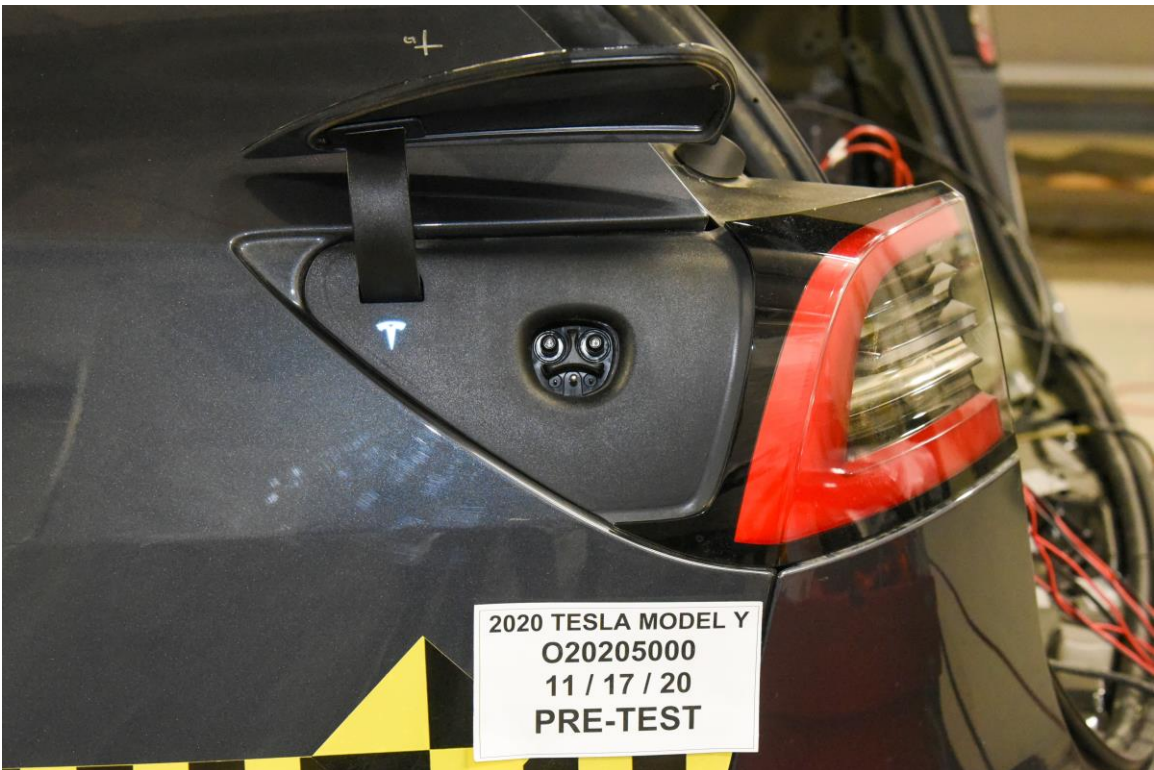
FIGURE 22. Pre-Test Fuel Filler Cap View
