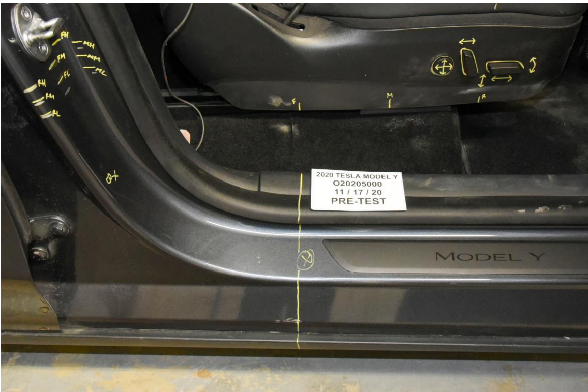
FIGURE 59. Pre-Test Passenger's Seat Fore-Aft Markings
