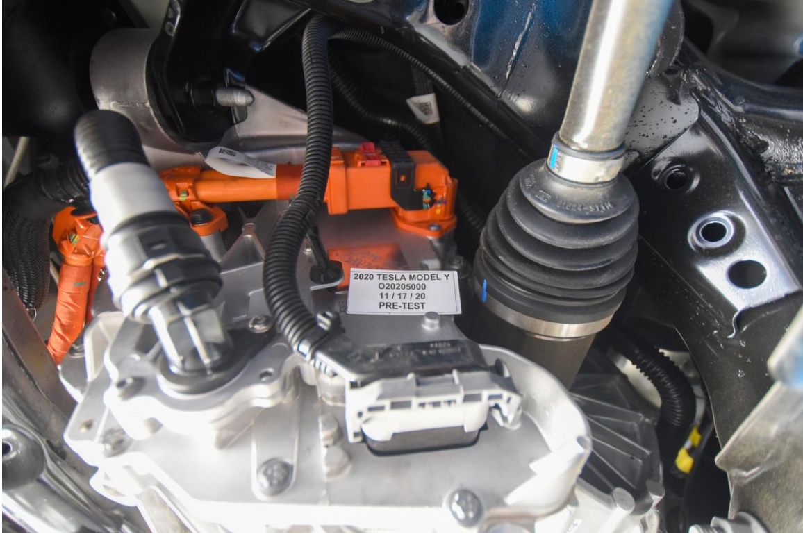
FIGURE 305-018a. Pre-Impact View of High Voltage Interconnect(s)
