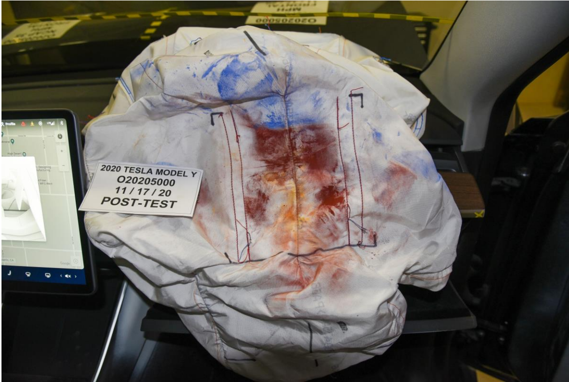
FIGURE 72. Post-Test Passenger Dummy Contact with Airbag
