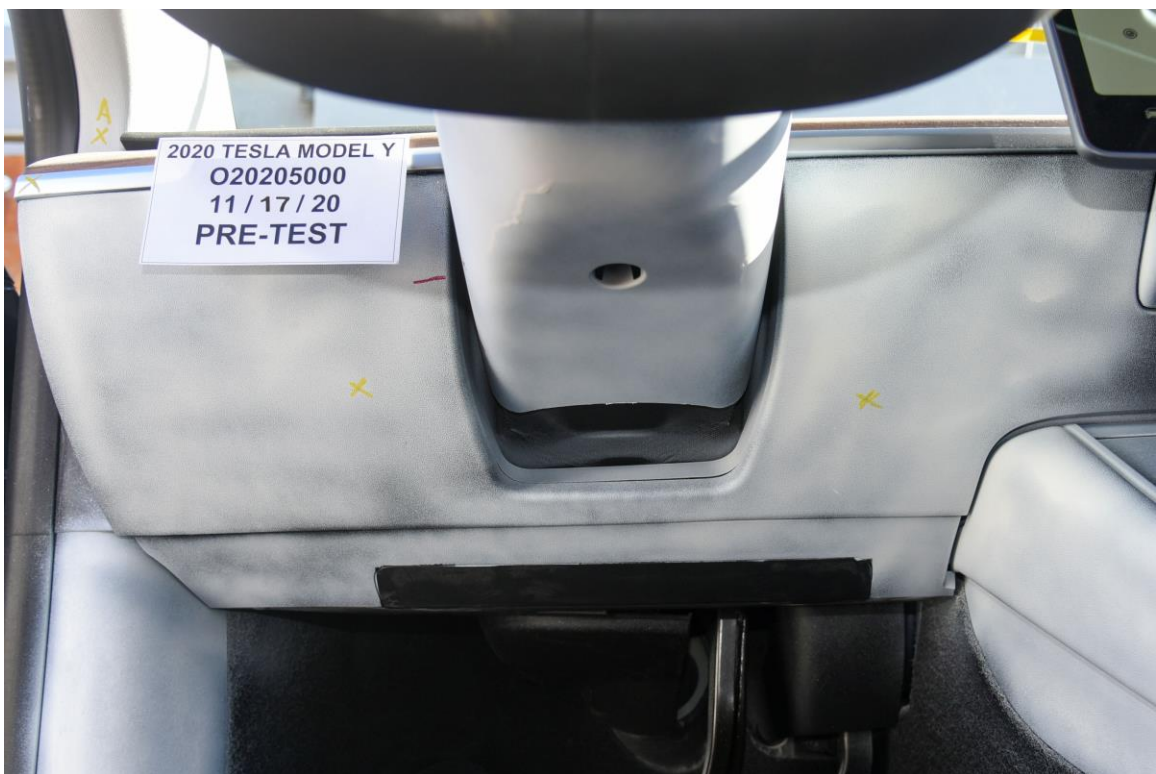
FIGURE 44. Pre-Test Driver's Side Knee Bolster (Incorrect Test Date; Should Read 11/17/20)
