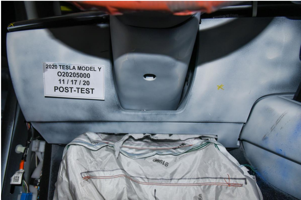
FIGURE 45. Post-Test Driver's Side Knee Bolster
