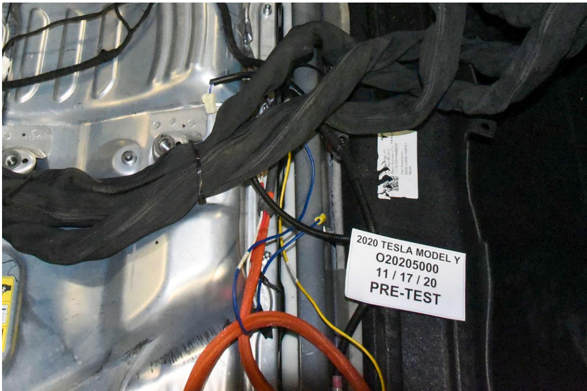
FIGURE 305-022. Pre-Impact View of High Voltage Leads Attached
