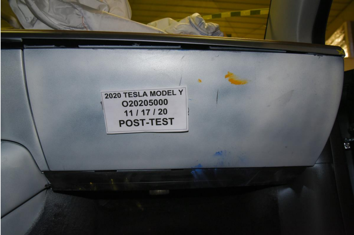
FIGURE 68. Post-Test Passenger's Side Knee Bolster
