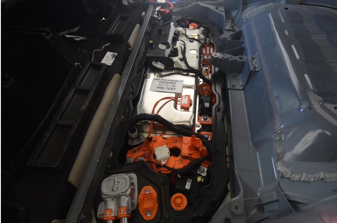
FIGURE 305-020. Pre-Impact View of Other Visible Electric Propulsion Components
