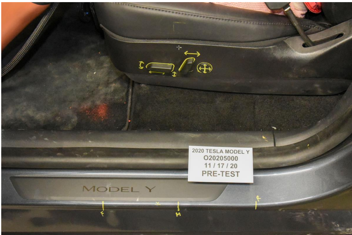
FIGURE 36. Pre-Test Driver's Seat Fore-Aft Markings
