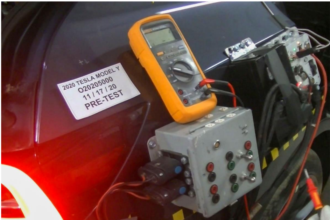
FIGURE 305-024. Pre-Impact View of Installed Test Interface Port
