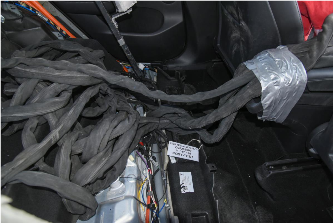
FIGURE 29. Post-Test Dummy Cable Routing
