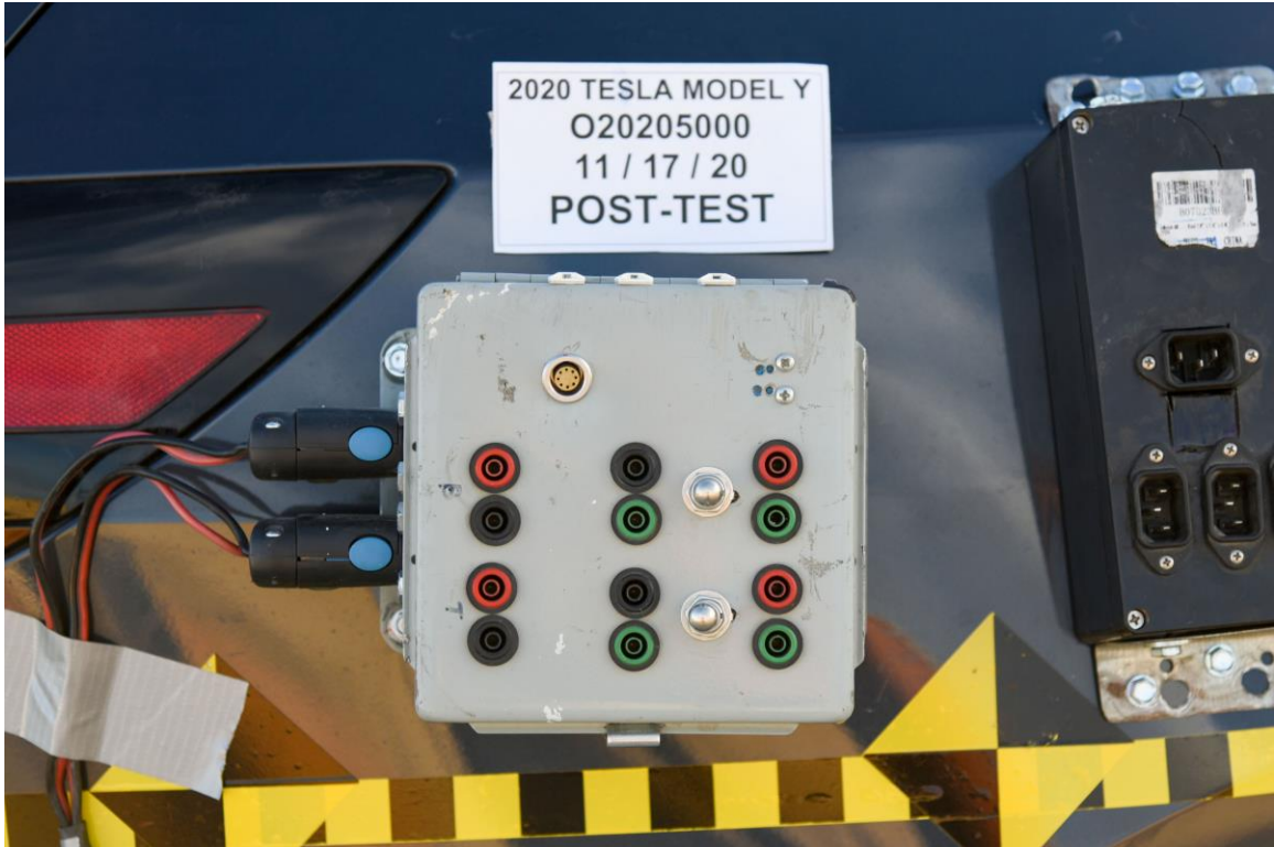
FIGURE 305-025. Post-Impact View of Installed Test Interface Port
