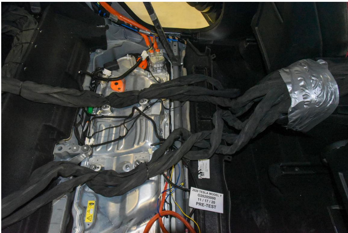
FIGURE 28. Pre-Test Dummy Cable Routing
