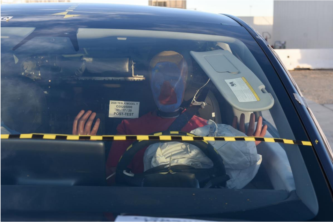
FIGURE 31. Post-Test Driver Dummy Front View
